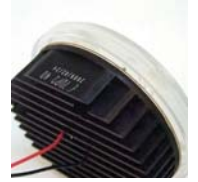
PCB with integrated heat sink.
