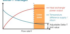
If cooling or heating coils are operated at an excessively high flow rate and thus at an excessively low differential temperature, above a certain operating point the energy consumption of the pumps and of the cooling and heat generators will rise - without increasing the power output.
